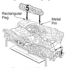
Figure 26 - Installing Log # 5
