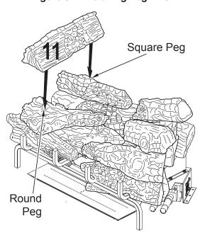
Figure 32 - Installing Log # 11
