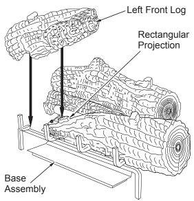
Figure 37 - Installing Left Front Log
