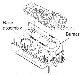
Figure 22 - Installing Log # 1
