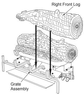
Figure 36 - Installing Right Front Log
