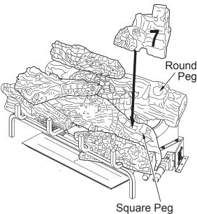
Figure 28 - Installing Log # 7
