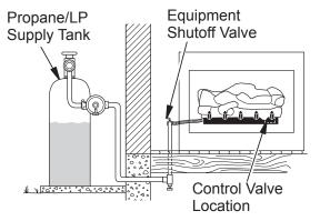
Figure 15 - Checking Gas Joints (Propane/LP Only)
