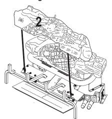
Figure 23 - Installing Log # 2
