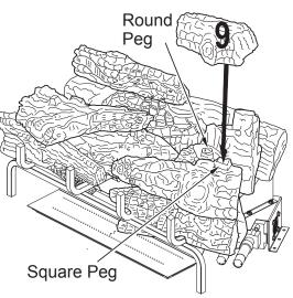
Figure 30 - Installing Log # 9
