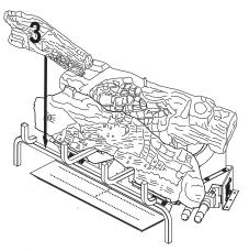
Figure 24 - Installing Log # 3
