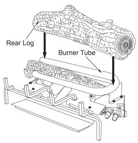
Figure 35 - Installing Rear Log
