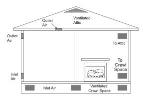
Figure 3 - Ventilation Air from Outdoors
