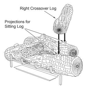
Figure 38 - Installing Right Crossover Log
