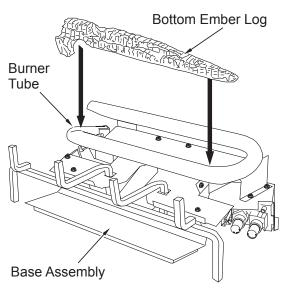
Figure 34 - Installing Bottom Ember Log
