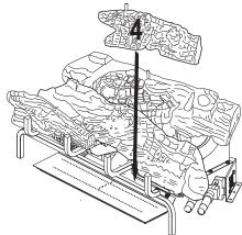
Figure 25 - Installing Log # 4
