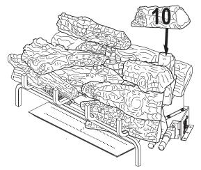
Figure 31 - Installing Log # 10
