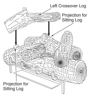
Figure 39 - Installing Left Crossover Log
