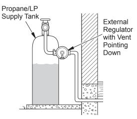
Figure 12 - External Regulator With Vent Pointing Down
