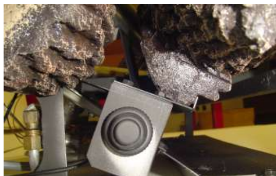
Figure 24A - Installing Front Left Log Side View
