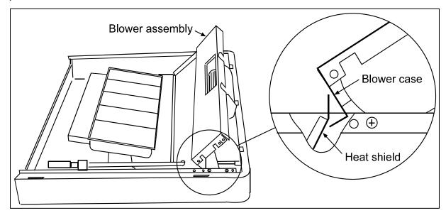
9. Lower the blower into the heater and secure both ends with sheet metal screws.
