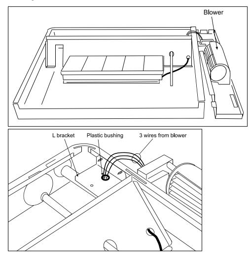
7. Make electrical connections shown in the diagram below
