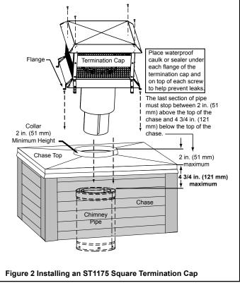
**Note:** The ST1175 is designed for use with the SL1100 Series pipe.
