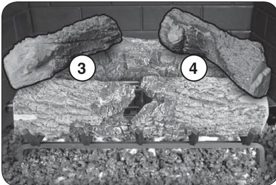
Place the left and right middle logs (logs #3 & #4) as shown.
