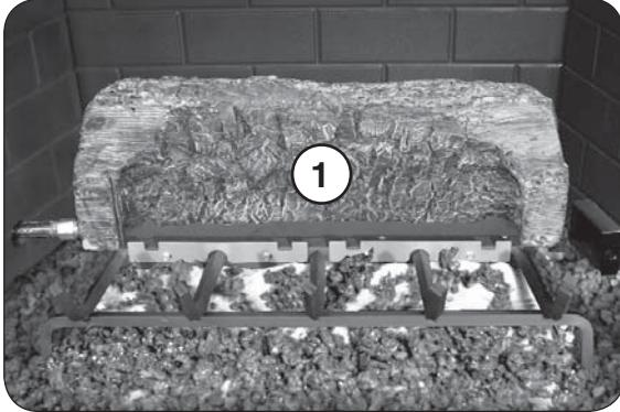
Place the rear log (log #1) as shown. The log should be slid back on the burner until it hits the backstop.
