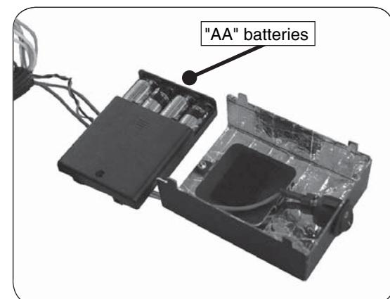
Fig. 20-3 Switch box batteries
