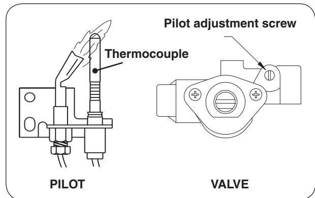
**Fig. 29-1** Pilot adjustment detail
