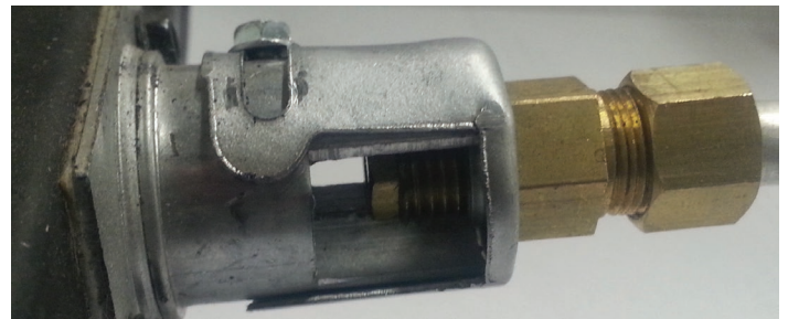
Figure 3 - Air Shutter Fully Open
