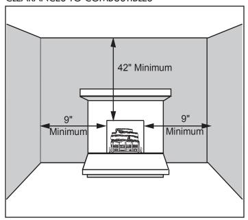
**Back Wall Clearance** — The appliance may be placed against a combustible back wall.
