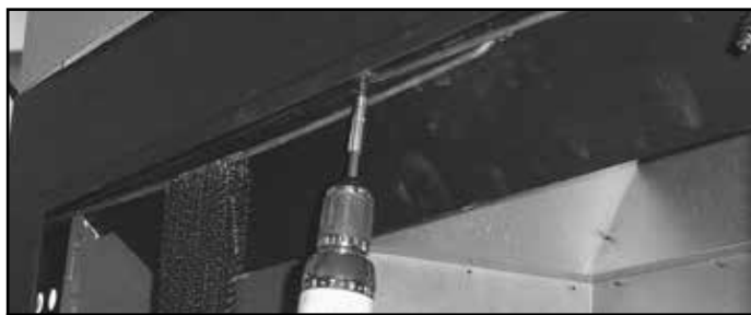
Figure 3.8 Removing the Screen Rods
