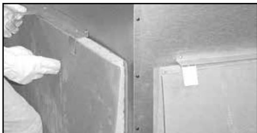
Figure 3.5 Unpacking Back Refractory
