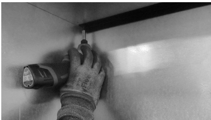
Figure 7.2 - Remove Rear Black Magic Glass Bracket
