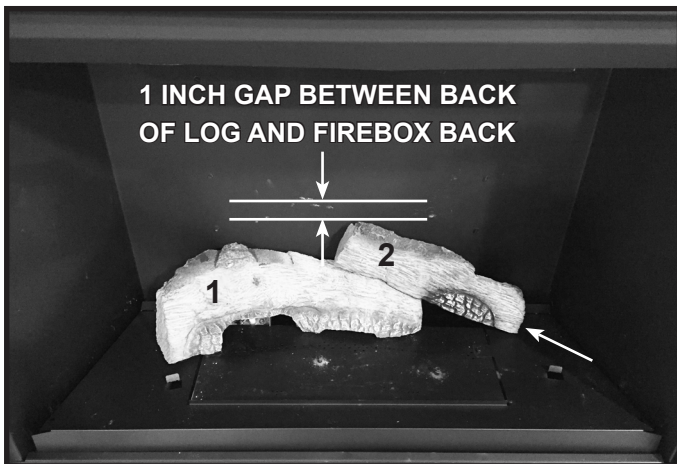
Figure 5. Install Right Rear Base Log
