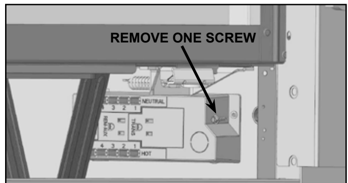
Figure 8.3 Junction Box Detail - JADE32IN-B
