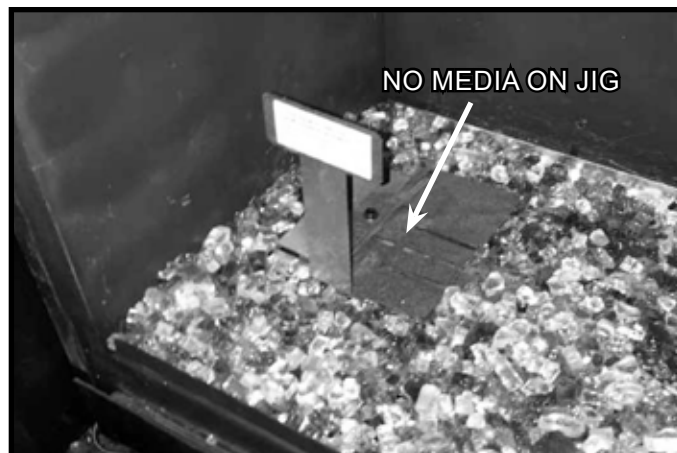
Figure 2. Media Placement Jig in Place
