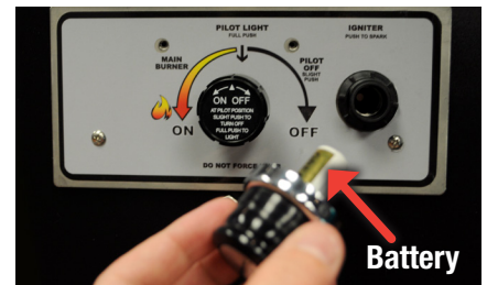
Figure 10.6 – Slide battery into spark igniter unit.
