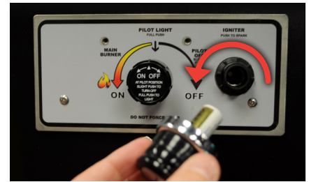
Figure 10.4 – Unscrew spark igniter unit cap.
