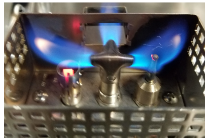
Figure 10.2 – Pilot flame coverage of thermocouple.
