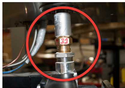
Figure 10.1 – Locating orifice for cleaning
