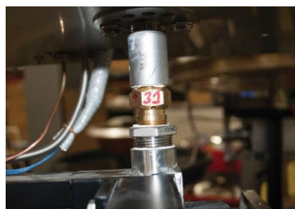
Figure 10.1 – Locating orifice for cleaning
