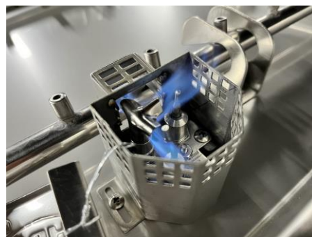
Figure 10.2 – Pilot flame coverage of thermocouple.
