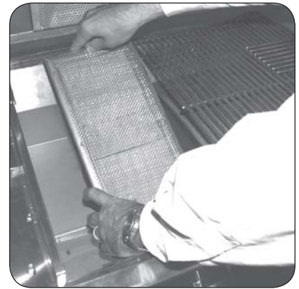
Fig. 4-2 Install new burner
