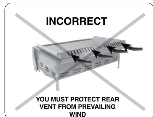
Fig. 12-4 Airflow direction - INCORRECT
