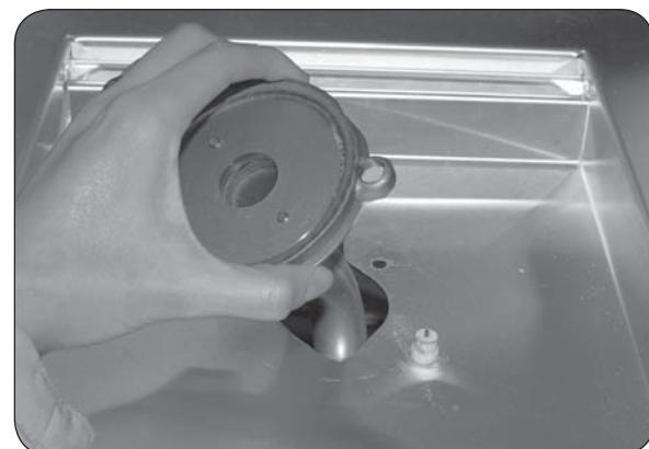
**Fig. 24-2 Remove burner**
