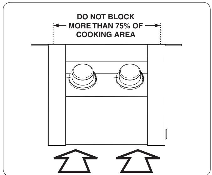
Fig. 10-1 Ventilation Diagram
