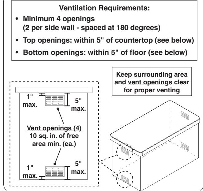
Fig. 11-1 Ventilation detail
