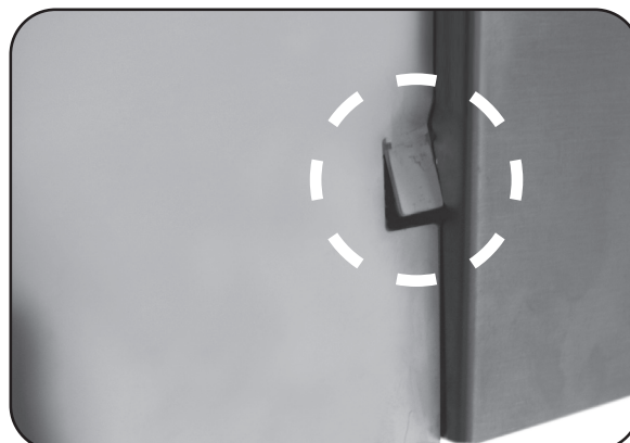
Fig. 26-3 Tab slightly bent in for clearance
