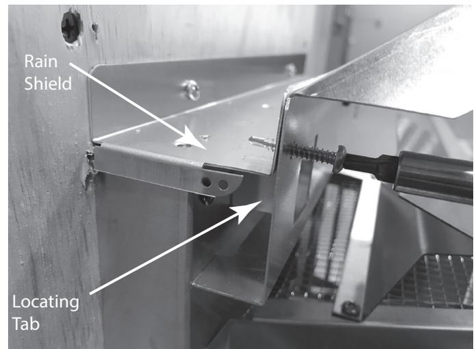
4. Lay bead of high temperature silicone in the channel between TRAP-VSS and cap rain shield to prevent water drainage between TRAP-VSS and rain shield.
