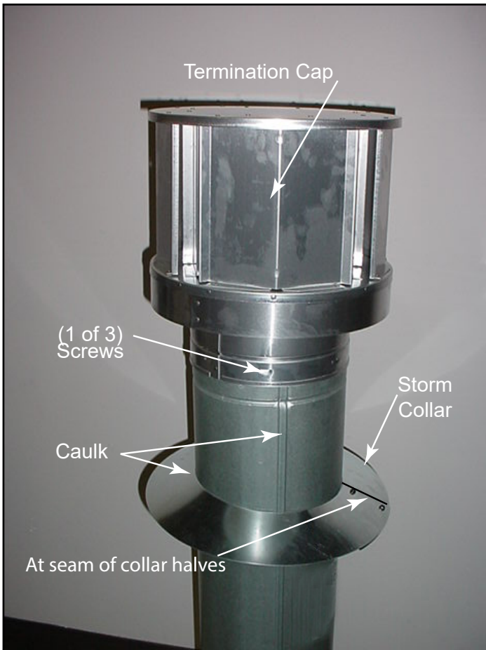
► Figure 20 Secure with Screws
