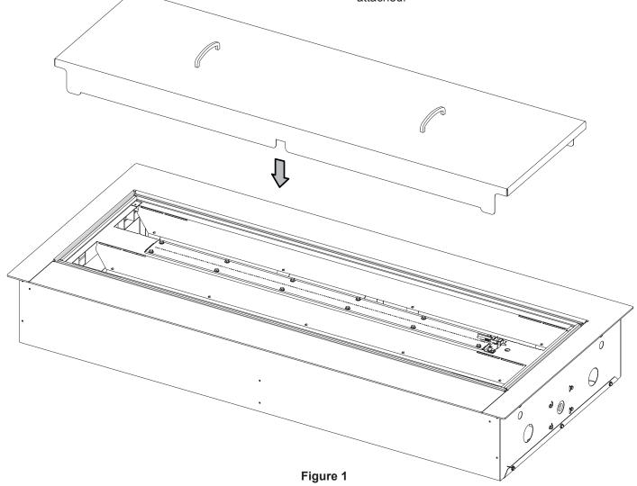
7. To install the weather cover, simply align the cover over the firepit as shown in **Figures 1 & 2.** The cover will nest to the outside of the filler trim pieces.
