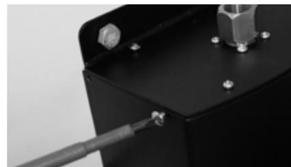
9. Fix Front cover to control housing using the 4xM4 screws provided.
