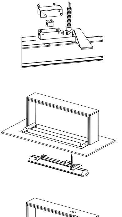
8. Rotate the heater into horizontal position in the ceiling box & then lower down onto the ceiling frame.
