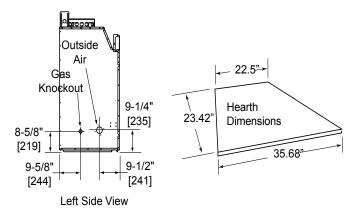
Framing dimensions in illustrations accommodate 1/2" finishing material.
