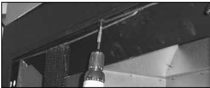
Figure 7.4 Removing the Screen Rods
