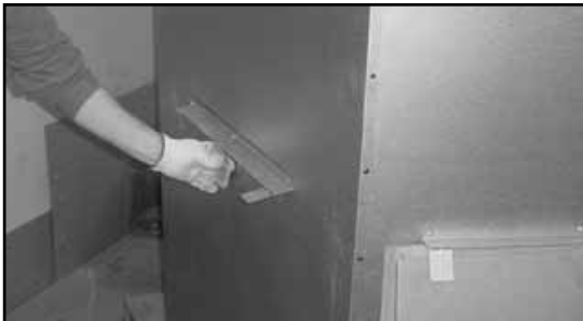
Figure 7.2 Bend Refractory Brackets Back Down
