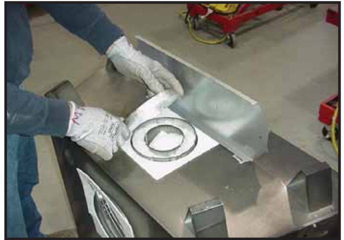
Figure 9.4 Remove the seal cap.
