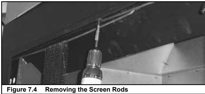
Figure 7.4 Removing the Screen Rods
