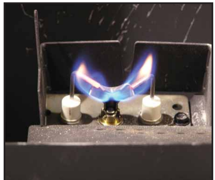
Figure 3.1 IPI Pilot Flame Pattern
