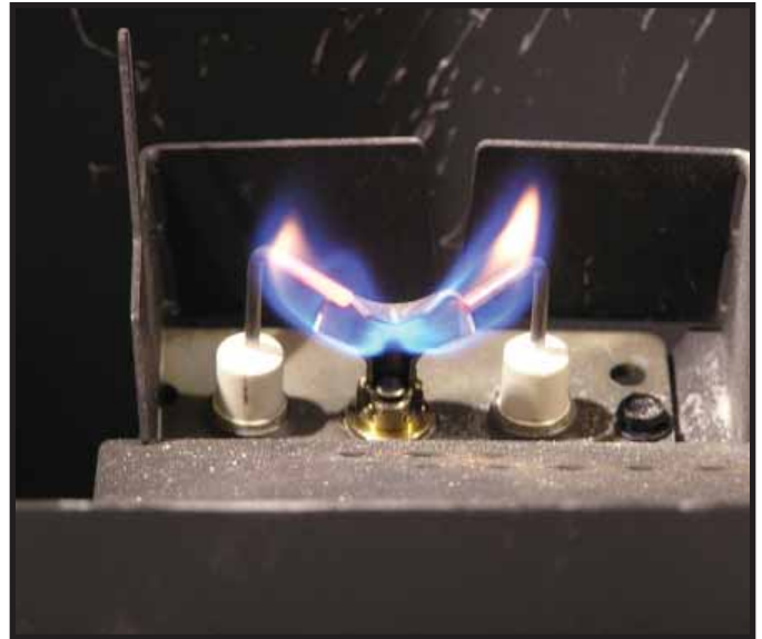
Figure 3.1 IPI Pilot Flame Patterns
