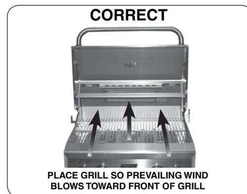
Fig. 10-3 Correct venting
