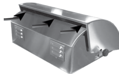
Fig. 12-2 Airflow direction - INCORRECT
