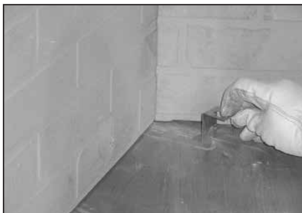
Figure 8.7 Slide Grate Retaining Bracket into Notch
