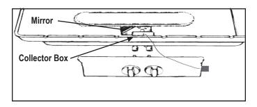
**A.** If there's a good spark, but the grill won't light, gas may not be flowing to the burner and into the collector box. The gas orifice or the venturi tube may be blocked. To clean, follow "Flashback" instructions.
