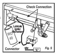
**B. Check spark**. Pull the connector wire from the collector box (see "X" *Fig. S*). Bring wire to bottom or top of control panel, hold about 1/8" away and operate the ignitor. Check for spark. If there is **no spark** replace the Rotary Ignitor. If there is **a spark** the Rotary Ignitor is OK, but the Collector Box/Electrode assembly should be replaced (the ceramic insulator could be cracked).
