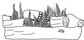
Figure 31 - Incorrect Flame Pattern
