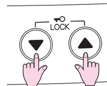
During normal operation the Function Lock may be activated and all controls other than the OFF switch will be locked. Deactivating the lock releases the controls. If the lock is activated while the heater is turned OFF, then all functions will be locked. If the heater is turned OFF while the Function Lock is activated, it cannot be turned ON again until the lock is deactivated.
