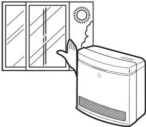
Keep away from flammable materials. Combustible materials must not be placed where the heater could ignite them. Do not place articles in front of the hot air discharge.
