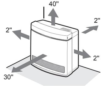
2. This heater may be installed on combustible flooring. When the heater is installed directly on carpeting, tile or other combustible material other than wood flooring, the heater shall be installed on a metal or wood panel extending the full width and depth of the heater.
