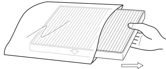
Note: Please turn off the "Air Purifier With Ion" button when replacing the HEPA filter.
