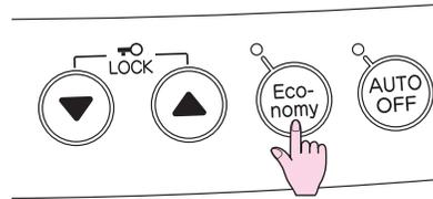
After the room is heated initially the air temperature may be dropped to a lower level without affecting comfort. 30 minutes after the selected room temperature (set with the thermostat) is reached, the Economy mode, if set, reduces the temperature by 2°F. After another 30 minutes it reduces the temperature by a further 2°F. This is an energy saving feature. The Economy mode does not operate if the heater is under capacity for the room size.
