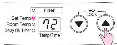
If the heater does not ignite then the pre-set temperature may not be set to a setting which is higher than the actual room temperature.
