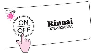
If the heater does not ignite on initial try, air may be remaining in the gas supply line. The spark generator will only continue for 30 seconds. After this, it will be necessary to press the ON/OFF button OFF, then ON again.
