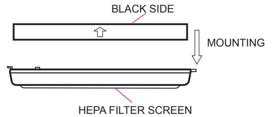
6. Install the HEPA Filter Screen into the appliance
