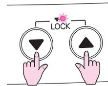
To deactivate the Function Lock simply press the "▼" and "▲" buttons at the same time for 2 seconds and the Function Lock indicator will go out.
