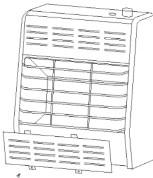
Figure 7 - Removing Lower Front Panel Of Heater
