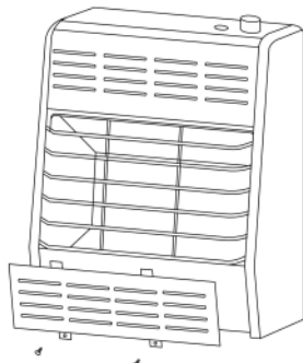
Figure 7 - Removing Lower Front Panel of Heater
