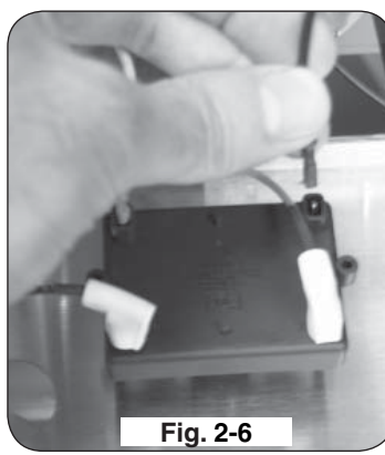
Connect wire to the ignitor module
